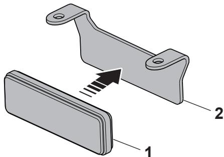
**GB** Remove the protective film and fix the reflector **1** on the kit bracket **2** as shown in the drawing.
