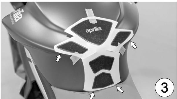
**GB** Keeping the protection kit in the previously established position on the tank, lift and cut the lower protective liner as indicated in figure 4.
