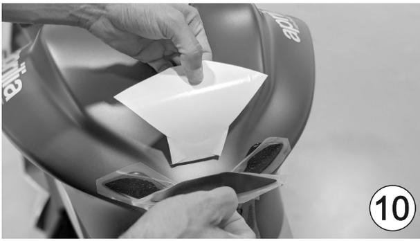
**GB** Gently lift the central upper part of the kit and remove the protective liner. Proceed with the relative application, paying attention to first stick the central area and then move on to the outer areas.
