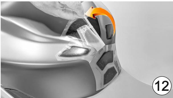
**GB** Make sure that all the various parts of the protection kit are well applied to the surface of the tank (there must be no air bubbles) and gently remove the protective film.
