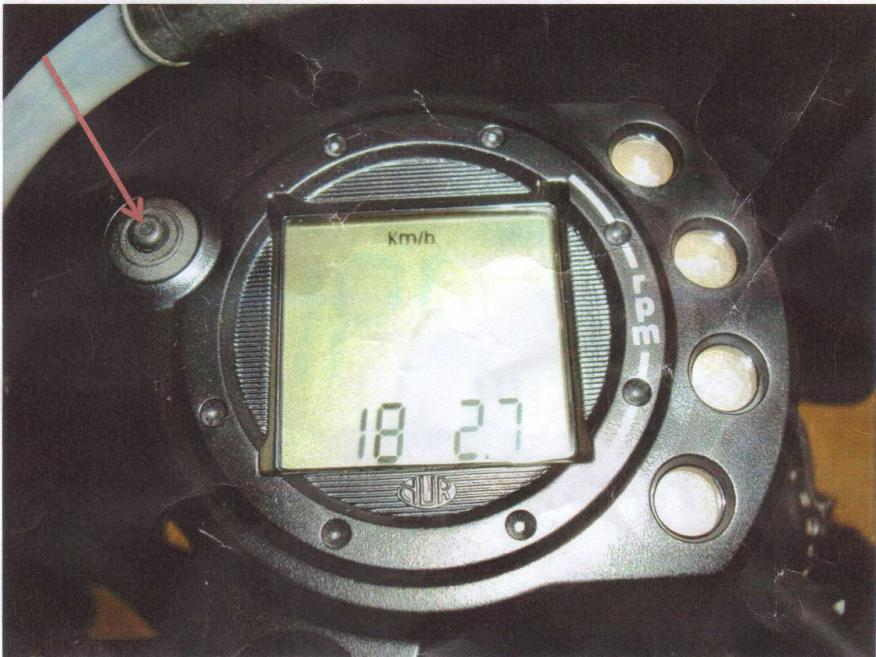
Once the correct size is selected hold this button for 3 seconds in order to memorize the selected wheel size.
